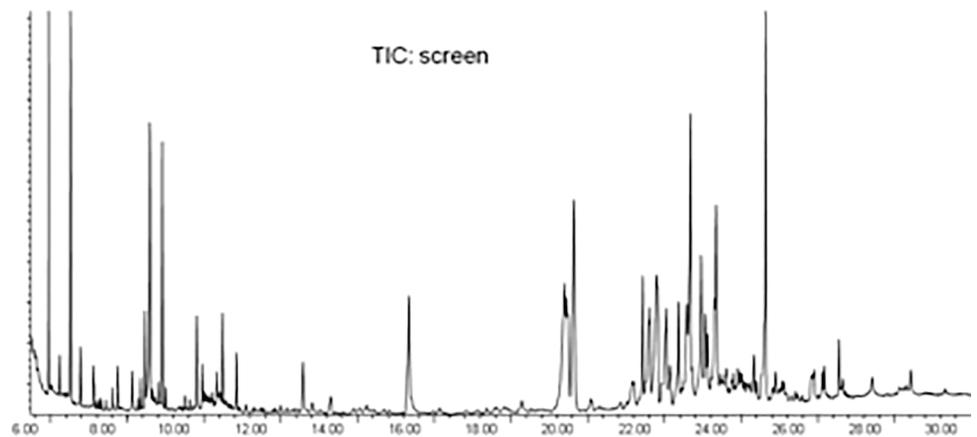
Figure 1 shows a typical GC-MS total ion chromatogram (TIC) of a simple ethanol extract from a sample of cartonboard used for food packaging. It shows a large number of peaks. Very few (if any?) of these peaks correspond to chemicals used in papermaking. So what are they? How does the responsible producer of the cartonboard or the responsible user (the food packer) check that they are all safe?
